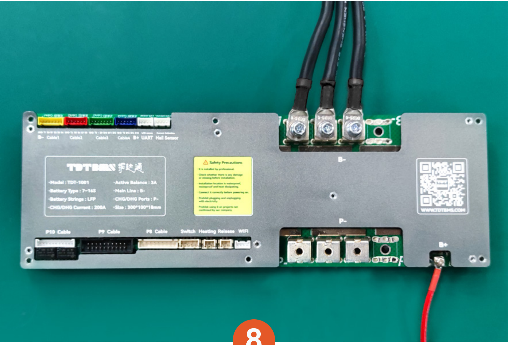
Connect the B- end of the BMS to the total negative terminal of the battery pack with thick silicone wires
